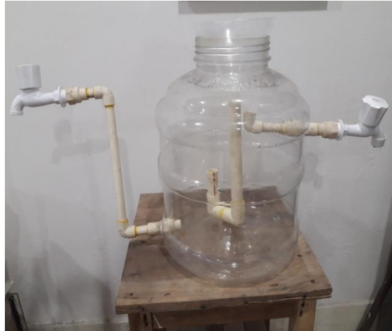
oil water separator for oil lighter than water
