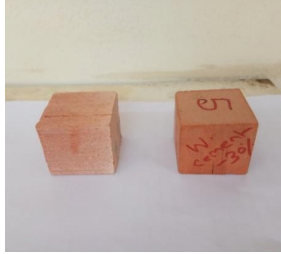
Fig 1: Prepared Refractory Sample(2in. x 2in. x 2in.)
