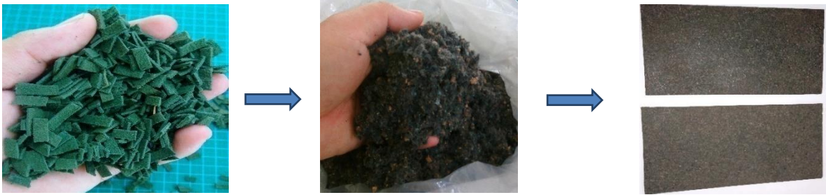
Picture: Leather board from waste leather
