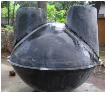
Fiberglass Biogas Plant
