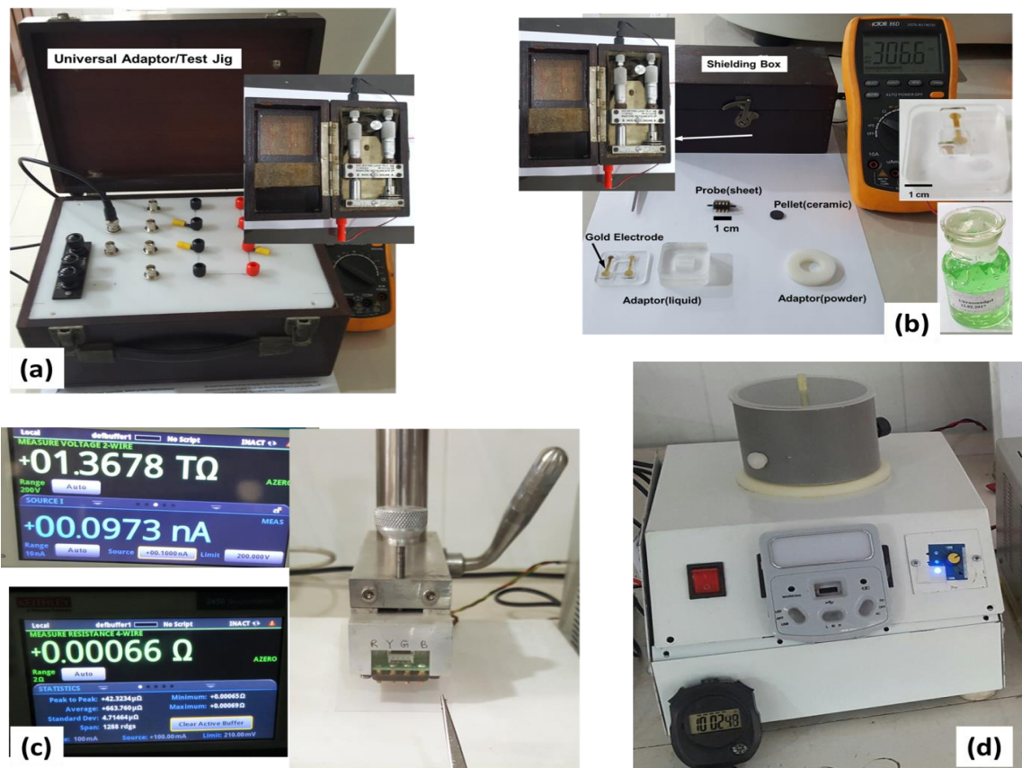
Figure 3: (a) Universal test Jig, (b) Adaptors for solid and liquid samples, (c) Sensitive Ultra-high and ultra-low resistivity measurement setup for thin and thick films, and (d) A preliminary designed proto-type portable (vacuum pump free) spin-coater for depositing conducting thin films.
