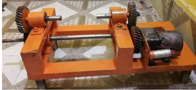
Picture: Shoe sole cleaning with polishing machine
