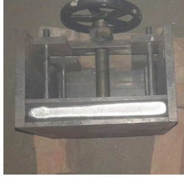
Fig: Pilot Plant Study for the recovery of Aluminium from E-waste ( Computer Hard Disks)
