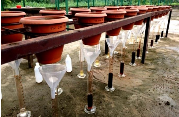
Figure: Collection of leachate from contaminated pots after extraction with HS
