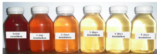
Waste water degradation of Industrial waste under open sunlight
