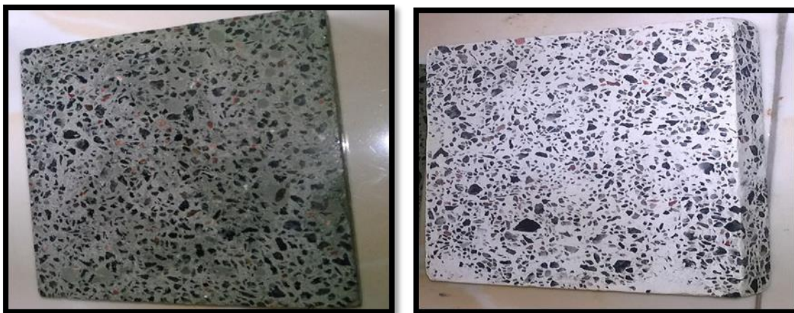
Fig: Pavement tiles using different wastes.
